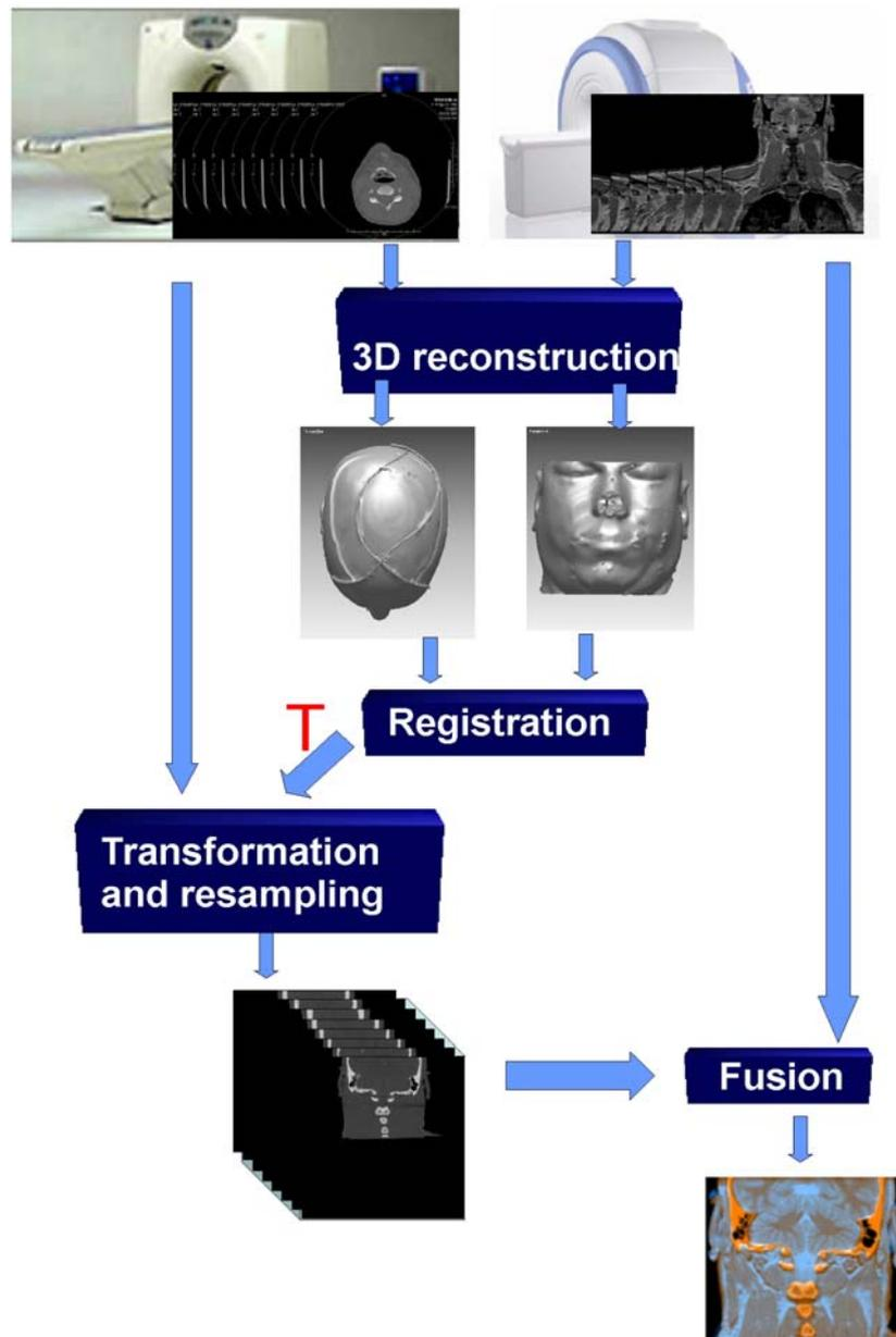
Fig. 1. The idea of the computer system of registration and fusion
