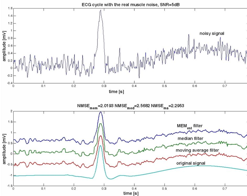
Fig.3 An example of filtering of ECG cycle corrupted with the muscle noise (upper plot) and results of filtering of various investigated filters (MEMest – MEM filter with  $\lambda'_{opt}$ , median – median filter, MAfilt – moving average filter, original – “clean” ECG cycle).
