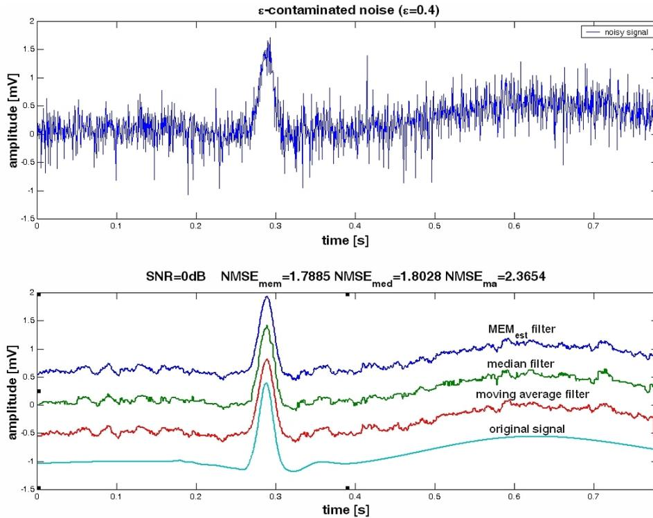
Fig. 2 An example of filtering of ECG cycle corrupted with  $\epsilon$ -contaminated noise (upper plot) and results of filtering of various investigated filters (MEMest – MEM filter with  $\lambda'_{opt}$ , median – median filter, MAfilt – moving average filter, original – “clean” ECG cycle).
