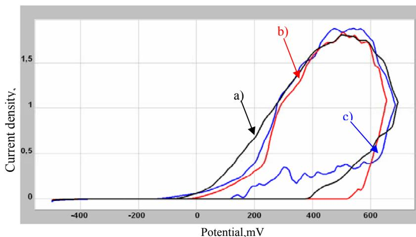
Fig. 13. The anodic polarization curve for plates used for 24 month: a) end side 1, b) middle side, c) end side 2
