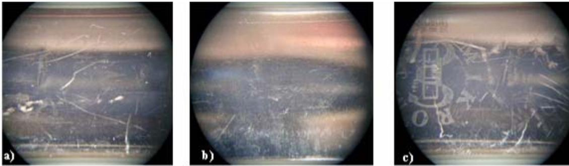
Fig. 11. Plate with the surface damage (26 month): a) end side 1, b) middle, c) end side 2
