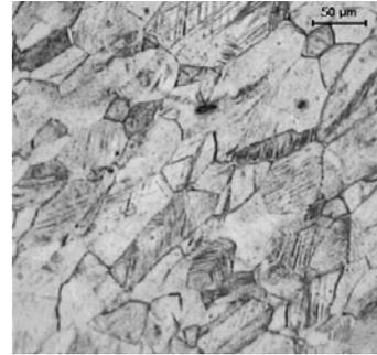
Fig. 8. Structure of the stainless steel in the maximum bent area, longitudinal microsection, magn. 200x
