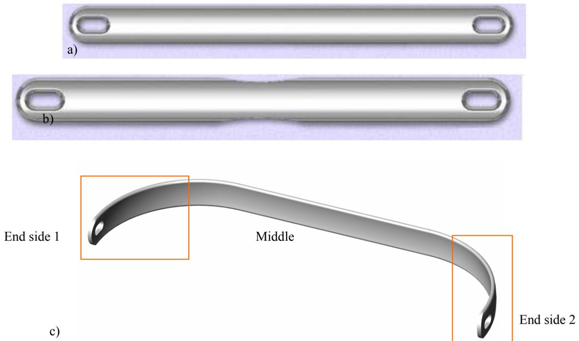
Fig. 2. Fixation plates: in initial state - a) narrow, b) wide [20], - c) after bending
