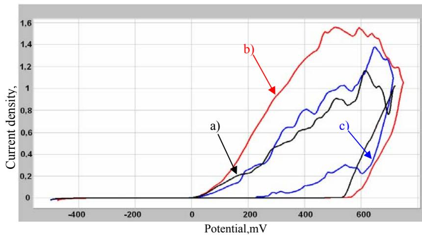
Fig. 15. The anodic polarization curve for plates used for 25 month: a) end side 1, b) middle side, c) end side 2
