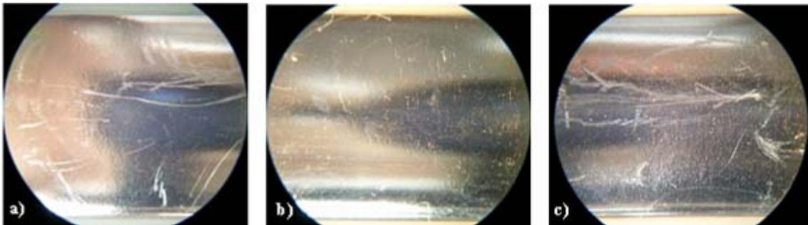
Fig. 9. Plate with the surface damage (24 month): a) end side 1, b) middle, c) end side 2
