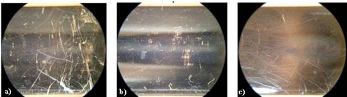
Fig. 10. Plate with the surface damage (25month): a) end side 1, b) middle, c) end side 2
