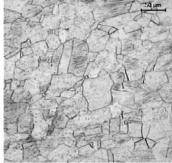
Fig. 7. Structure of the stainless steel, longitudinal microsection, magn. 200x
