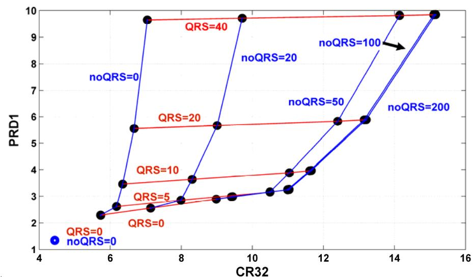
Fig.3. Correlation between achieved mean square error (PRD1) and compression ratio  $CR_{32}$  (related to 32 bit floating number) as a functions of percentage value of main threshold within and beyond the QRS complex (marked QRS and noQRS respectively).
