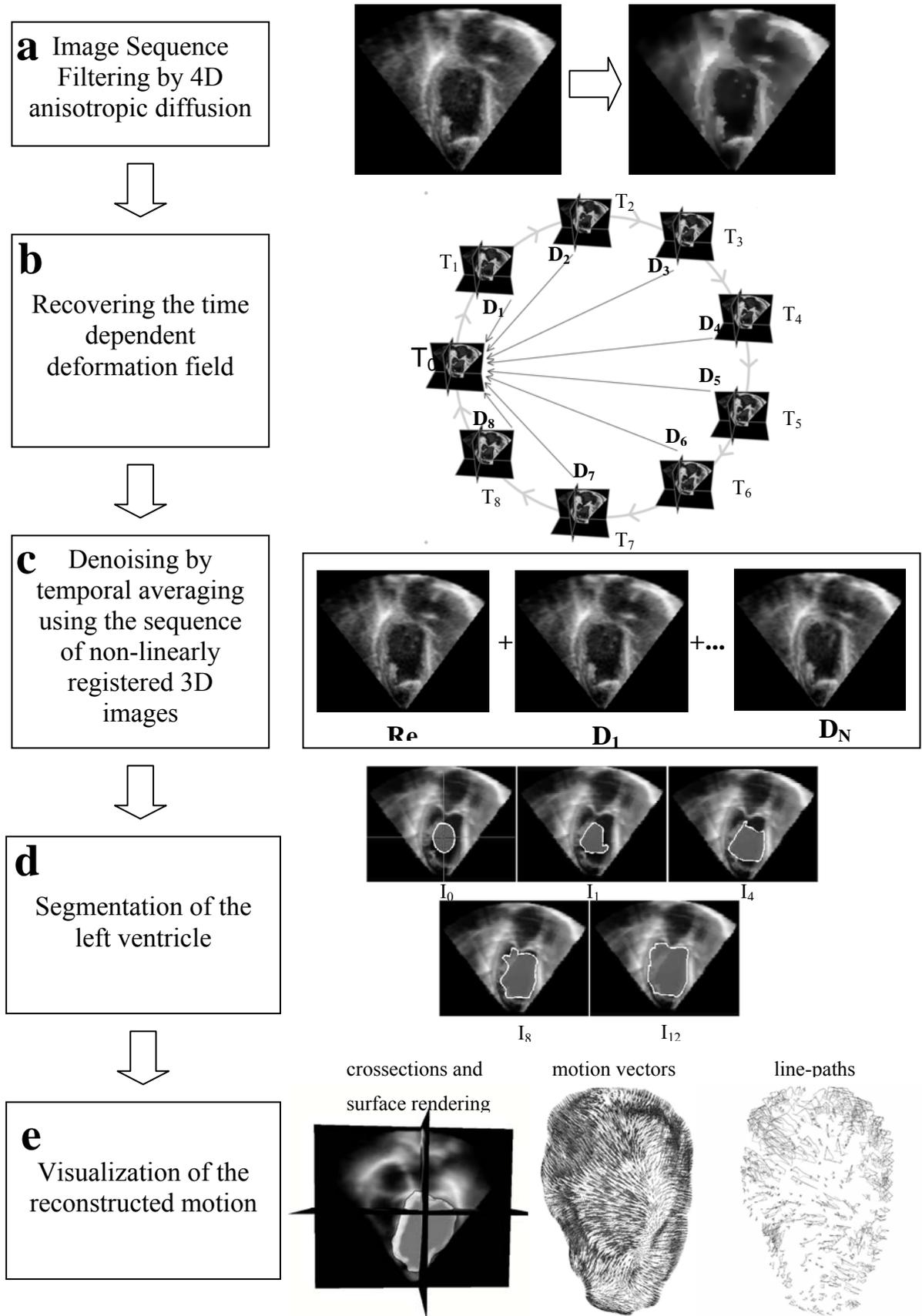
Fig.1. The flow diagram of our heart motion reconstruction algorithm.
