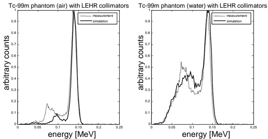
Fig.5. Simulated and experimental spectra of  $^{99m}\text{Tc}$  phantom with air and water filling and with LEHR collimators.
