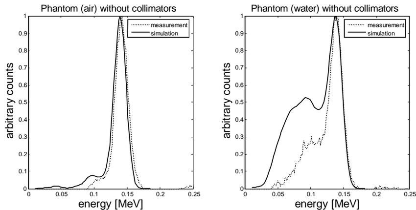
Fig.6. Simulated and experimental spectra of  $^{99m}\text{Tc}$  phantom with air and water filling and without collimators.
