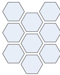
Fig.1. Collimator holes shape and configuration. Diameters of the hexagon and septa thickness depend on the collimator type.
