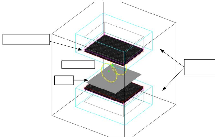
Fig.3. Gamma camera model visualization form GATE platform. Two heads are in starting positions (angle 0° for detector 1 and 180° for detector 2).
