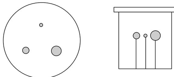
Fig.2. Phantom draft. Left: top view, right: side view. Grey spheres are filled with  $^{99m}\text{Tc}$  with constant concentration of the activity.
