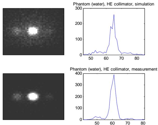
Fig.9. Phantom with water results for HE collimator. Up – simulation, down – experiment. Left: images obtained from the detector. Right: Profiles of the pixel intensity acquired for the spheres filled with the  $^{99m}\text{Tc}$ .
