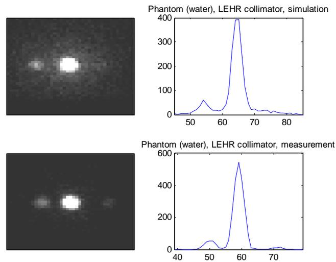
Fig.8. Phantom filled with water results for LEHR collimator. Up – simulation, down – experiment. Left: images obtained from the detector. Right: Profiles of the pixel intensity acquired for the spheres filled with the  $^{99m}\text{Tc}$ .
