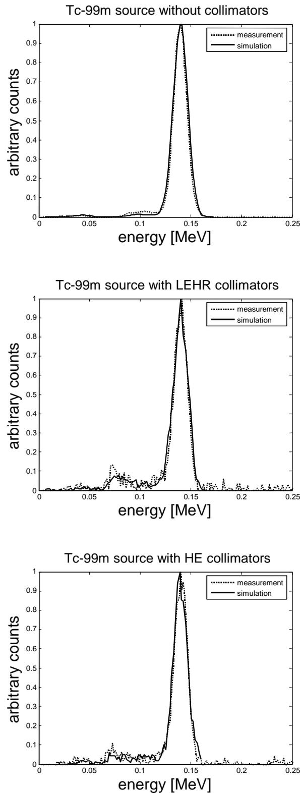
Fig.4. Simulated and experimental spectra of  $^{99m}\text{Tc}$  source in three configurations of the system: without collimators (up), with LEHR collimators (middle), with HE collimators (down).
