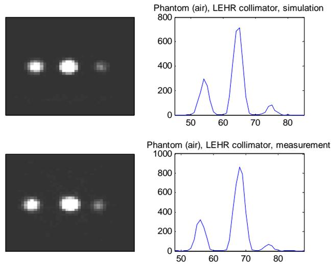
Fig.7. Phantom filled with air results for LEHR collimator. Up – simulation, down – experiment. Left: images obtained from the detector. Right: Profiles of the pixel intensity acquired for the spheres filled with the  $^{99m}\text{Tc}$  (x axis - pixel number, y axis - counts).
