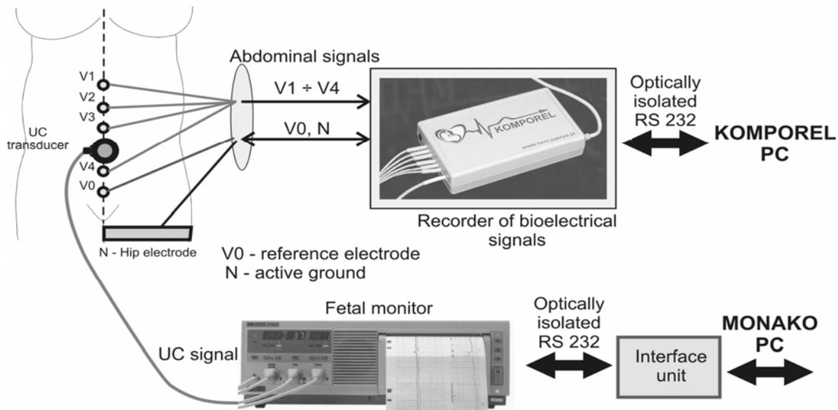
Fig.1. System for simultaneous recording of mechanical and electrical uterine activity.
