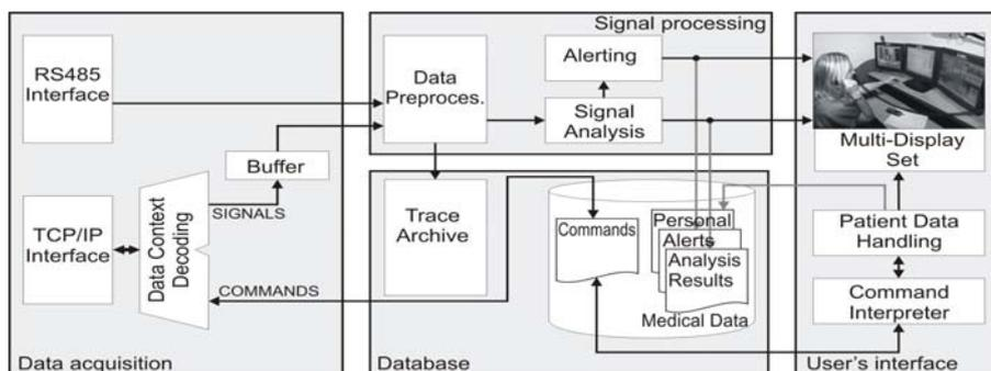
Fig.4 The structure and interactions between different components of the Surveillance Centre from the fetal monitoring system.
