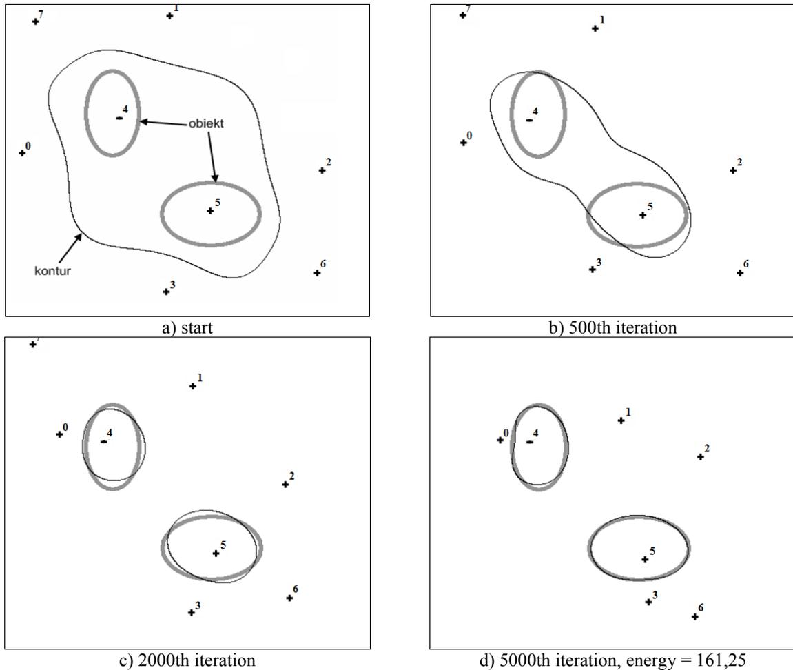
Fig.2. Adjustment of the contour to two disjoint objects
