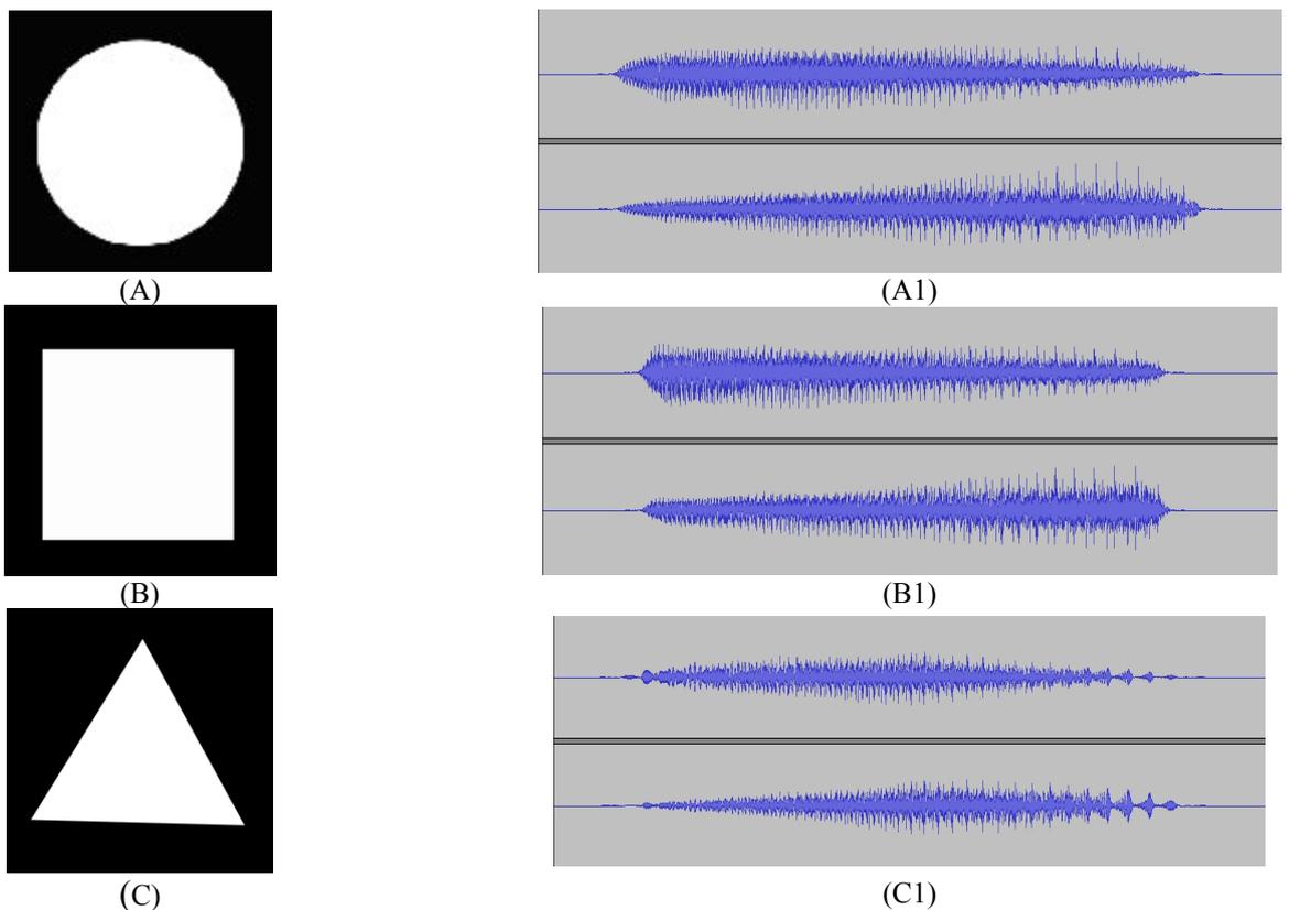
Fig. 3. Sample soundscape vocabulary generated by IS for basic shapes images. The standard shapes: circle (A), square (B) and triangle (C) are associated with different sounds, illustrated here as different stereo waveforms (A1), (B1) and (C1), respectively.
