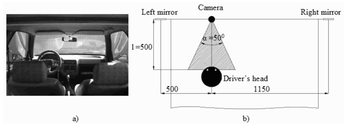
Fig. 3. The car's interior a) and the camera's localization b).
