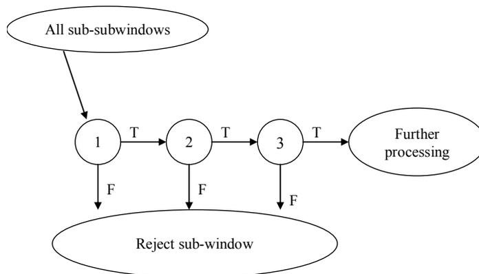
Fig. 6. The schema of the cascaded objects' detection
