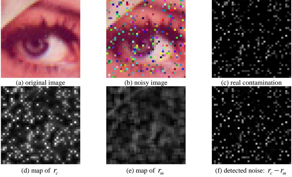
Fig. 3. Illustration of the noise detection scheme: test image (a), noisy image (b), injected impulse noise (c). Below the maps of  $r_c$ ,  $r_m$  and their difference  $r_d = r_c - r_m$  is presented (d-f)
