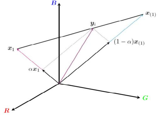
Fig. 2. Construction of the filter output as a weighted mean of the central pixel  $\mathbf{x}_1$  and vector median  $\mathbf{x}_{(1)}$ .
