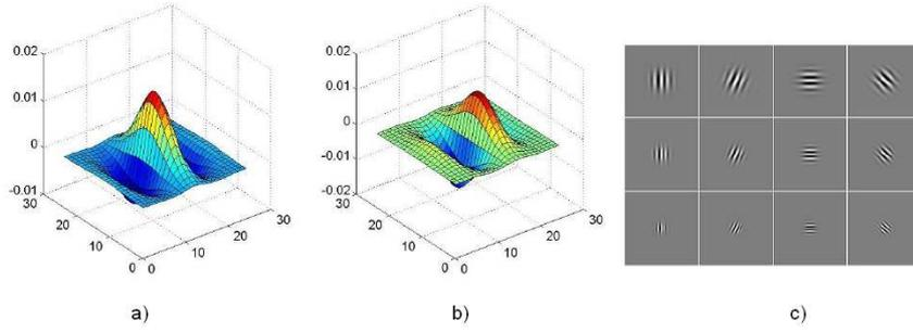
Fig. 5. Real (a) and imaginary (b) parts of Gabor wavelets and Gabor kernels with different orientations (c)
