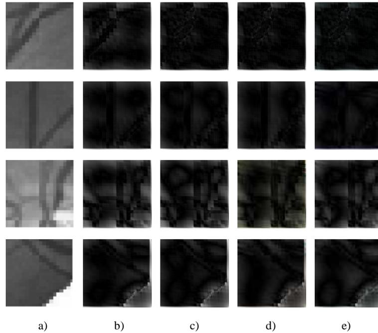
Fig. 7. Original block retina image (a) and real part of  $Gab(x; y; \theta)$  for  $\theta = 0$  (b),  $\theta = 45$  (c),  $\theta = 90$  (d),  $\theta = 135$  (e)
