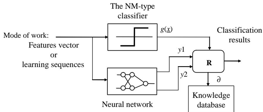
Fig. 3. Scheme of the hybrid recognition system. (Description of elements is presented in the text below)
