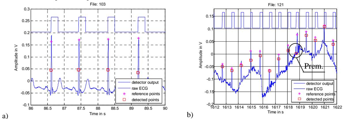
Fig. 6. Sample detection results: a) – high quality signal, b) – baseline drift
