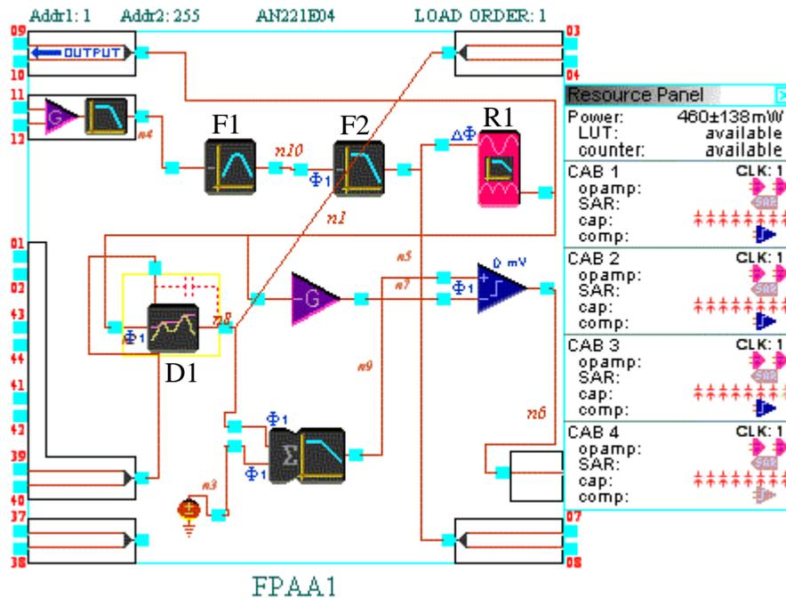
Fig. 3. The schematic of the QRS detector
