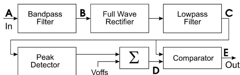
Fig. 1. Classical hardware QRS detector – block diagram [1]
