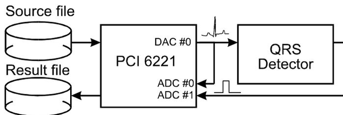
Fig. 5. Test workbench – block diagram
