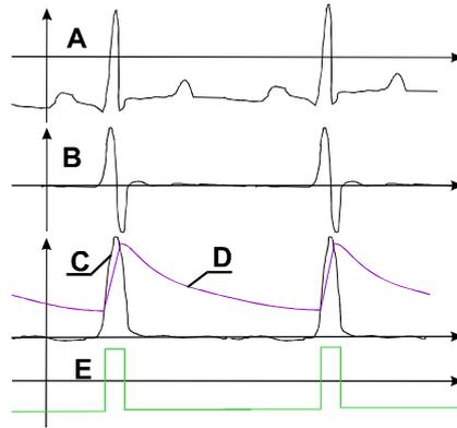
Fig. 2. Waveforms in important nodes of the hardware QRS detector
