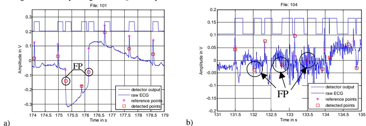
Fig. 7. Sample detection results: a) – baseline step change, b) – high frequency noise
