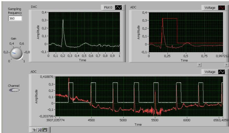
Fig. 4. Screenshot of the virtual instrument for ECG output and data acquisition
