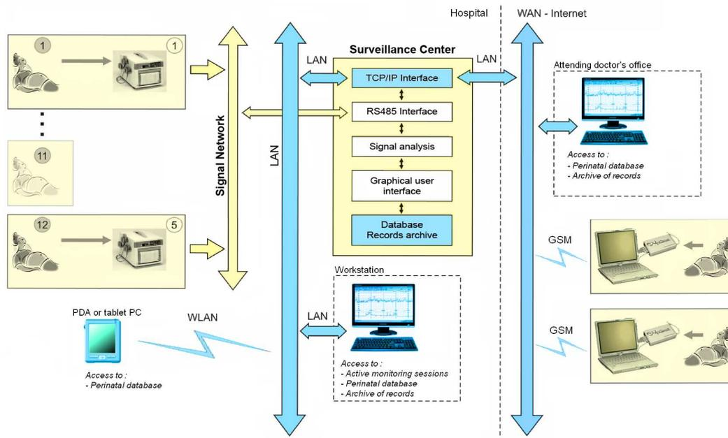
Fig. 1. A structure of centralized fetal monitoring system incorporating remote devices as well as classic bedside monitors located in hospital
