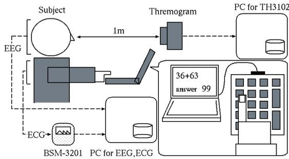
Fig. 1. Measurement system
