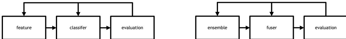
Fig. 3. Comparison of classical pattern recognition system design and MCS design.
