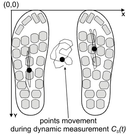
Fig. 7. Movement of the points  $C_s(t)$ ,  $C^L(t)$  and  $C^R(t)$  during dynamic measurements.
