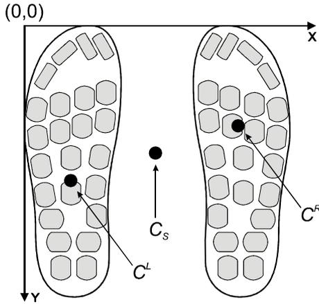
Fig. 6. Displacement of the points  $C_s$ ,  $C^L$  and  $C^R$  in the static measurement.
