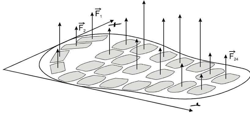
Fig. 5. The forces  $\vec{F}_i$  hooked in the  $C_{P_i}$  points [1]
