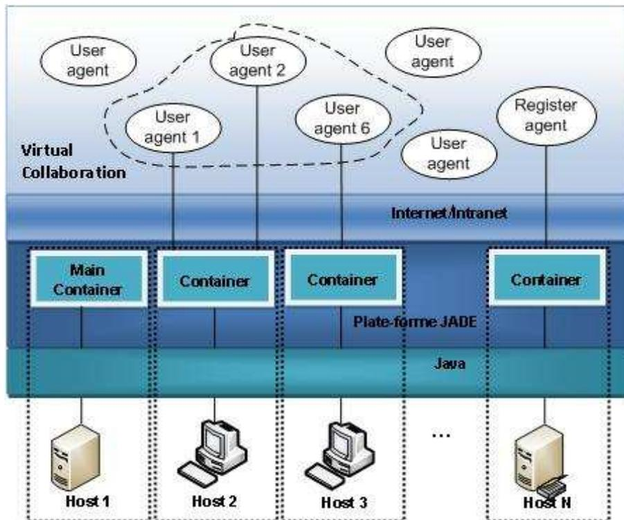
Fig. 4. Implementation of architecture using JADE.
