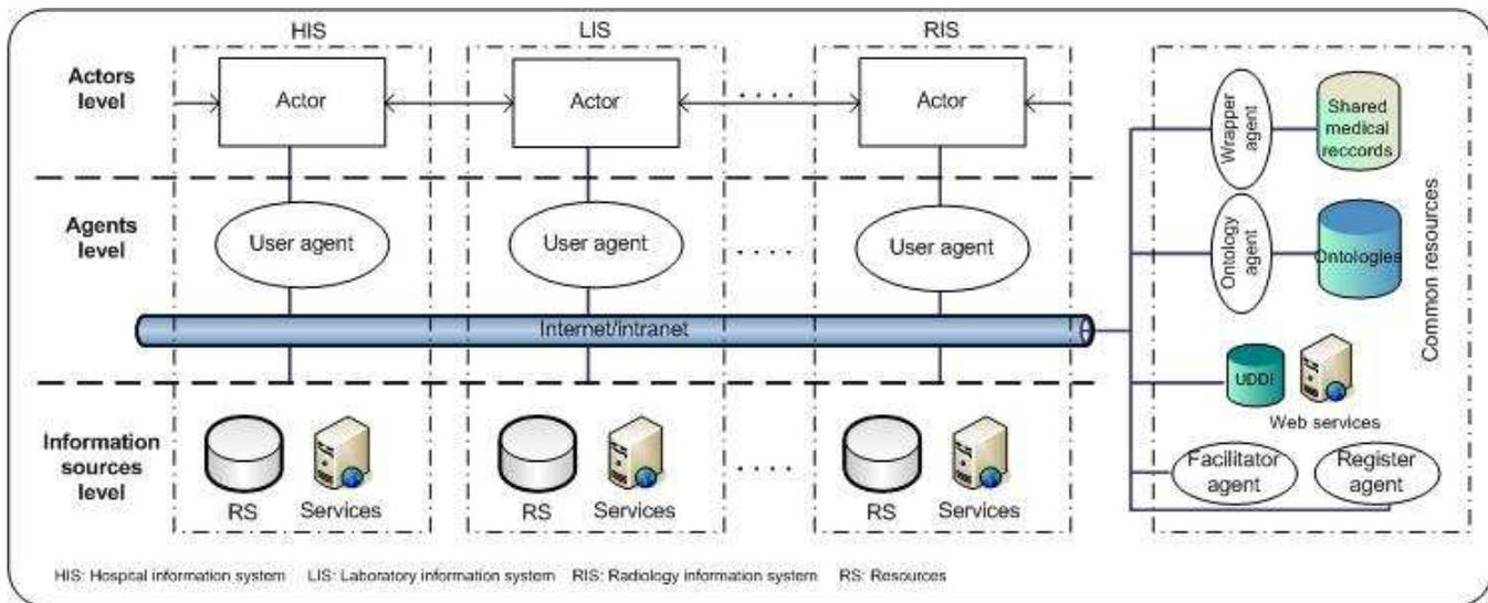
Fig.1. DAMIS: an agent based architecture for the MIS.
