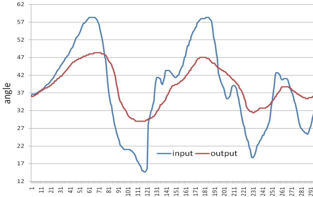
Fig. 3. Phase shift appears in relation to actual angle.
