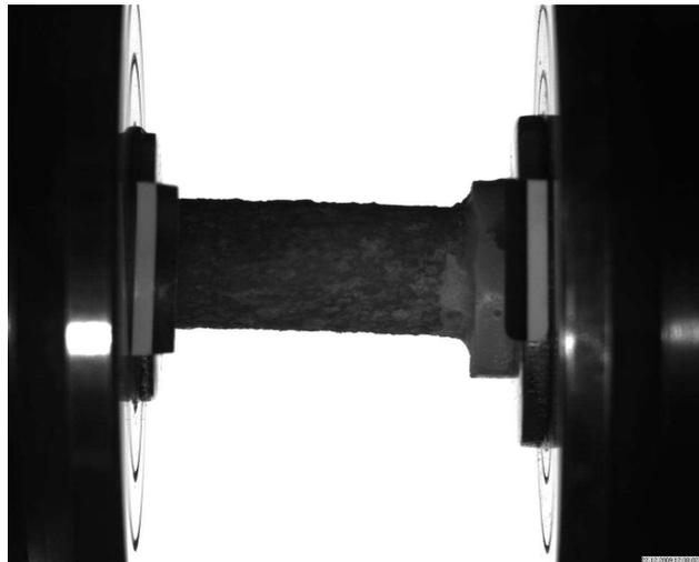
Fig. 4. The sample with the setup to compression test monitored by video extensometer.
