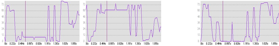
Fig. 4. Different Kohonen winning neuron contours for the same utterance. Right-most result is obtained using modified algorithm therefore silence is always placed in or near 0-th neuron. (Y axis: winning neuron, X axis: the time). In this example Kohonen network was of the size 8x9 giving 72 neurons.
