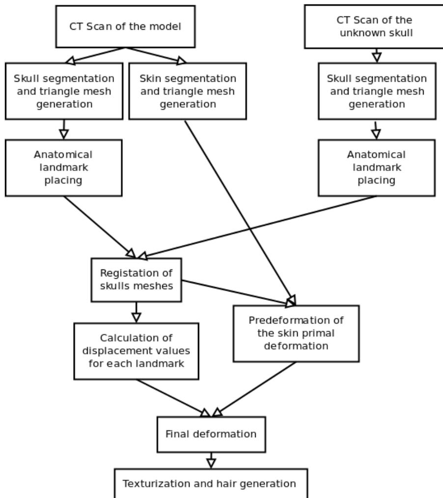
Fig. 1. General workflow of the reconstruction procedure.
