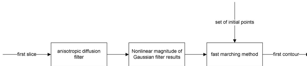
Fig. 2. Scheme of the initial contour segmentation for threshold level set method.
