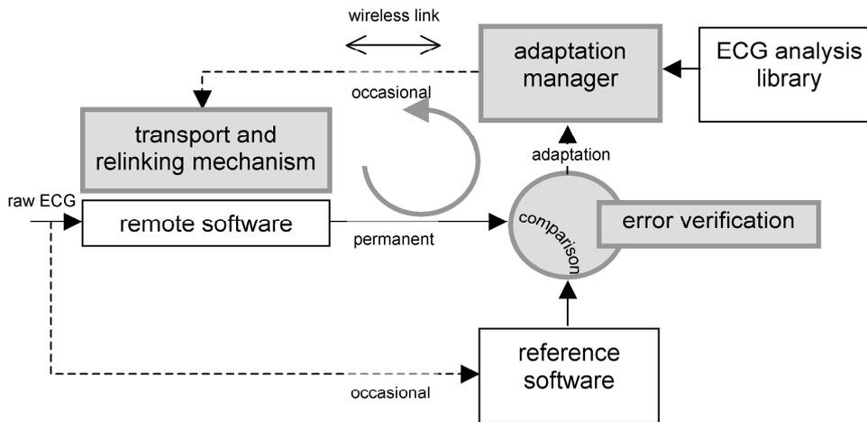
Fig. 1. Block diagram of the autoadaptive system for ubiquitous cardiology.
