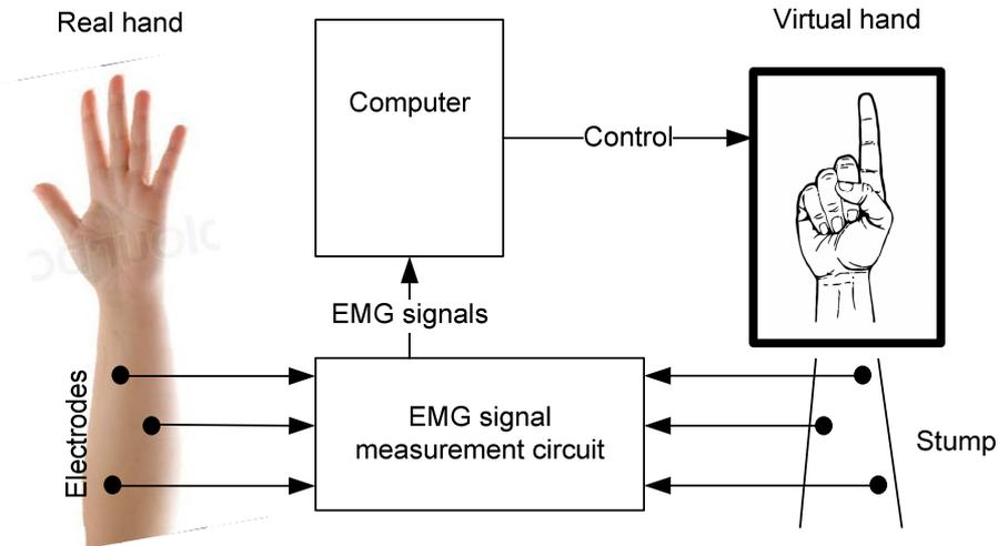
Fig. 6. The block diagram of the measurement system for identifying the relation between the hand movement and EMG signal taken from the muscles of forearm and stump.
