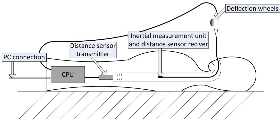
Fig. 5. Block diagram of TEE simulation device.
