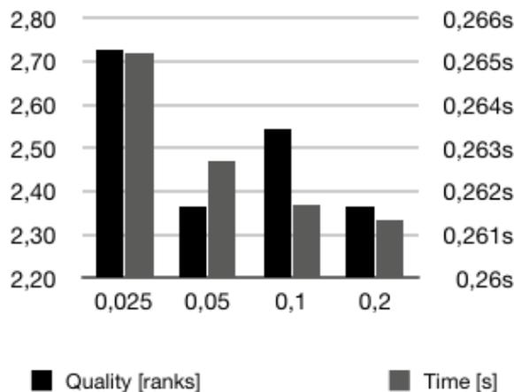
Fig. 1. Comparison of classification time and classification accuracy of DES-DT system for different values of parameter  $r$ .
