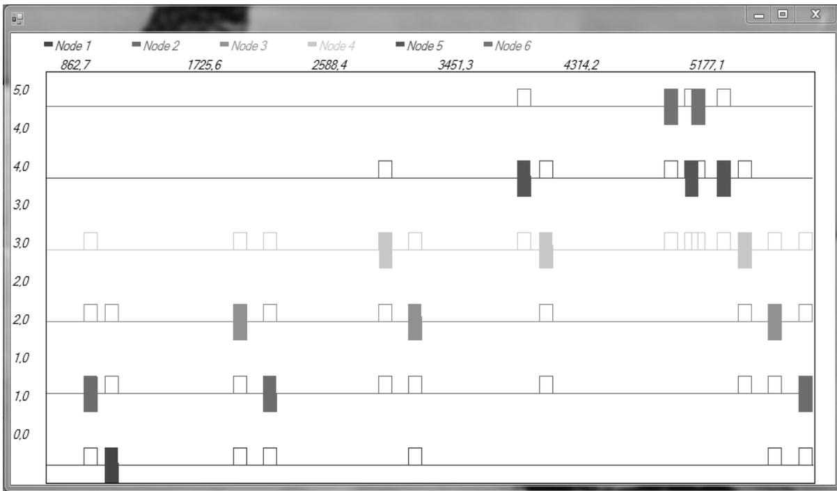
Fig. 4. Activity of wireless stations during the network configuration procedure, followed by normal operation when collected data is successively transmitted toward the central station.
