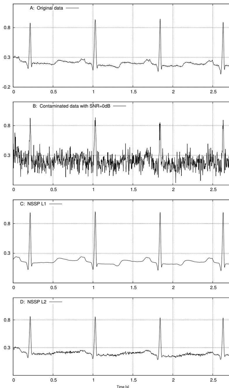
Fig. 2. Noise reduction on an electrocardiogram. A: the original signal, B: the contaminated signal with SNR=0dB. C: The filtered signal obtained with the proposed method. D: The filtered signal obtained with the reference method. The embedding dimension is  $m = 110$ .
