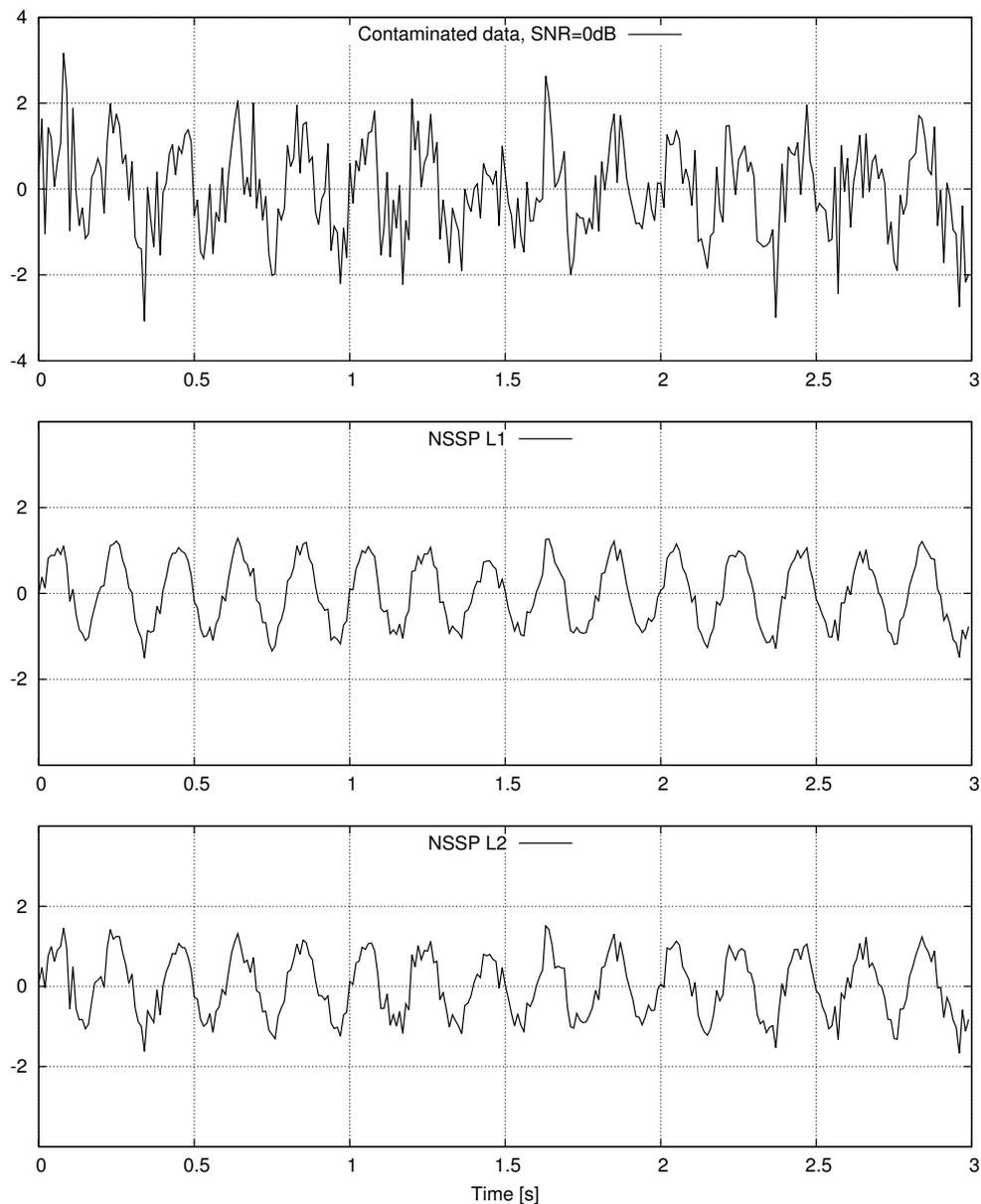
Fig. 1. Noise reduction of an analytical signal. Upper: the sinusoidal signal with the amplitude  $1V$  and the frequency  $f = 5Hz$ . Middle: the test signal after nonlinear filtering with the proposed method. Lower: the test signal after filtering with the reference method. The embedding dimension is  $m = 30$ .
