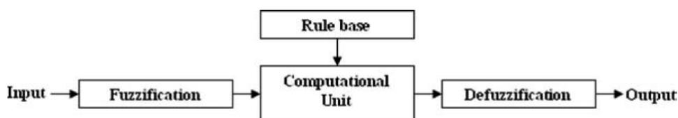
Fig. 1. Fuzzy Controller Architecture.
