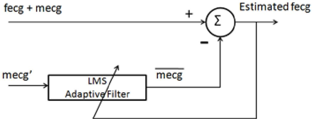
Fig. 3. Principle of the adaptive filter used.
