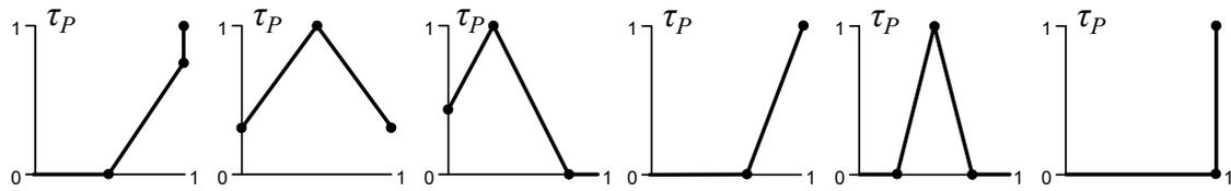
Fig. 3. Sample triangular truth functions and nodes needed to describe them.
