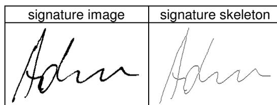
Fig. 2. An example of a signature and its thinned version.
