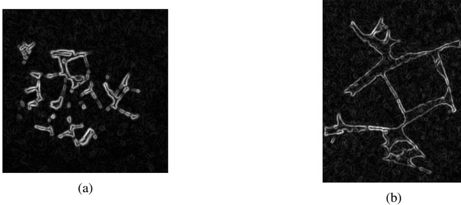
Fig. 7: Canny-Deriche edge detection gradient magnitude: image containing small objects (a), image containing big objects (b).
