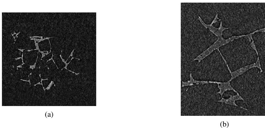
Fig. 5: Image after histogram normalisation: image containing small objects (a), image containing big objects (b).
