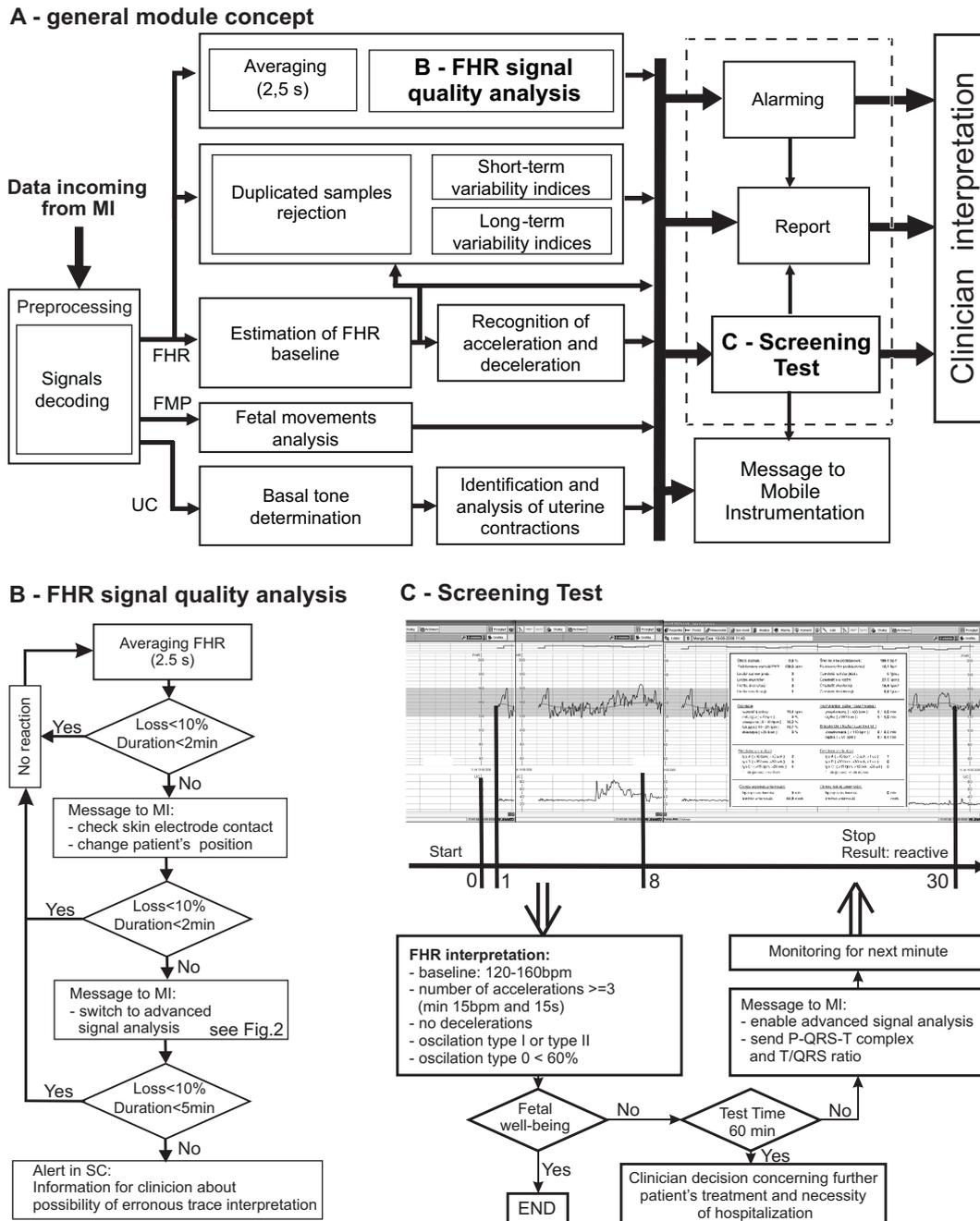
Fig. 3. Basic components of the Surveillance Center module responsible for analysis of signals obtained from MIs: A general module concept, B smart selection of the analysis algorithms for MI using the FHR signal quality data, C Screening test for fetal well-being during pregnancy.
