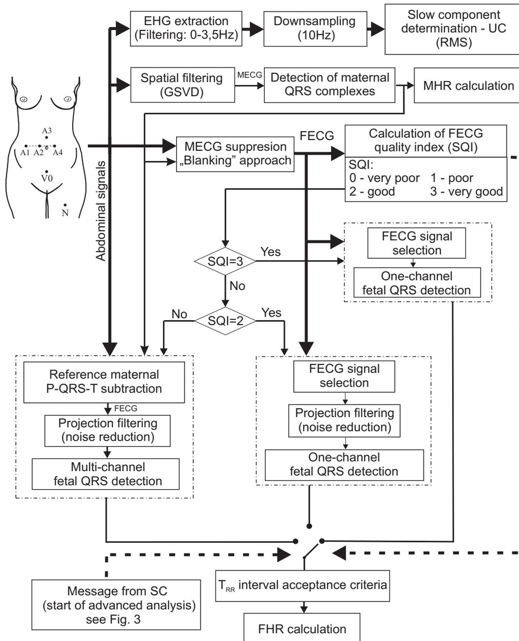
Fig. 2. Smart selection of biosignal analysis algorithms in the Mobile Instrumentation controlled directly by MI using the FECG quality index SQI.
