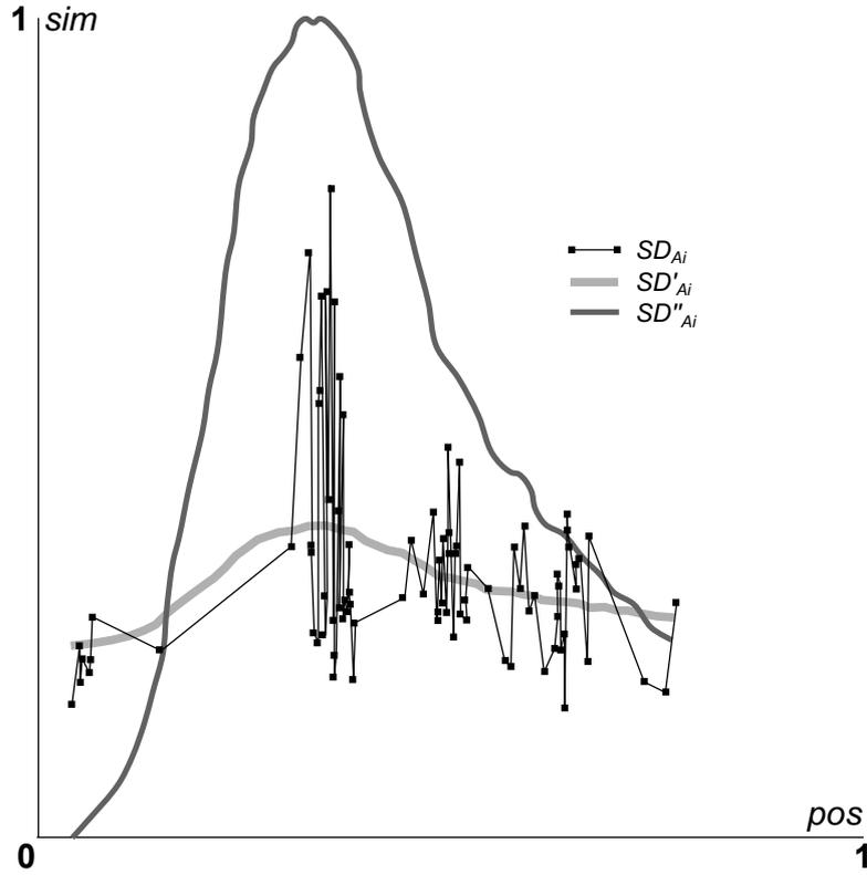
Fig. 2. Fuzzy set obtained from similarity distribution of one sample window compared with 9 other signatures of the same person. Black squares connected with thin black lines represent original values ( $SD_{A_i}$ ). The thick lightgray line represents softened version of the original chart using arithmetic average ( $SD'_{A_i}$ ). The thick darkgray line is the softened version after normalization ( $SD''_{A_i}$ ).
