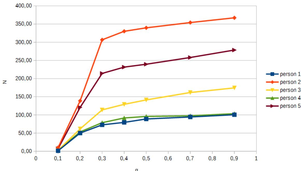
Fig. 4. Average number of filtered windows according to maximum level of  $\alpha$  (trigger). Results obtained for signatures of 5 different individuals.
