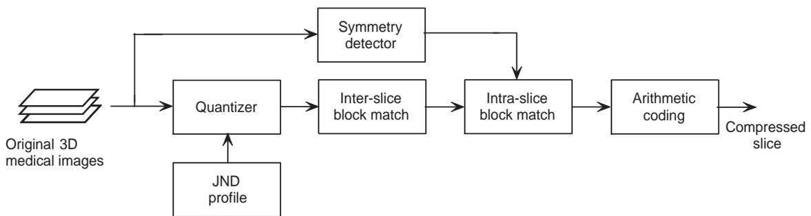
Fig. 4. Block diagram of perceptually lossless image compression with symmetry.
