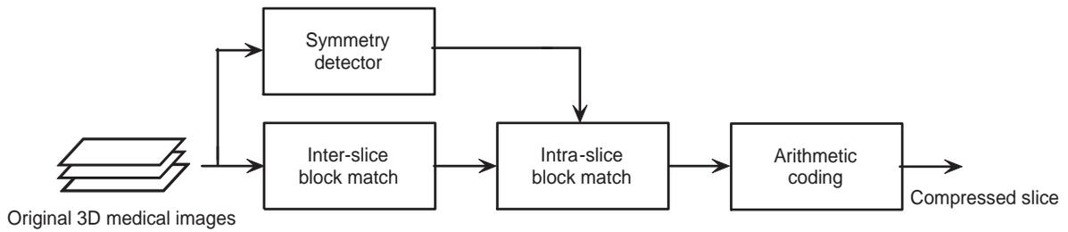
Fig. 3. Block diagram of lossless image compression with symmetry.
