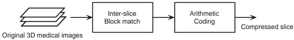
Fig. 1. Block diagram of lossless image compression.
