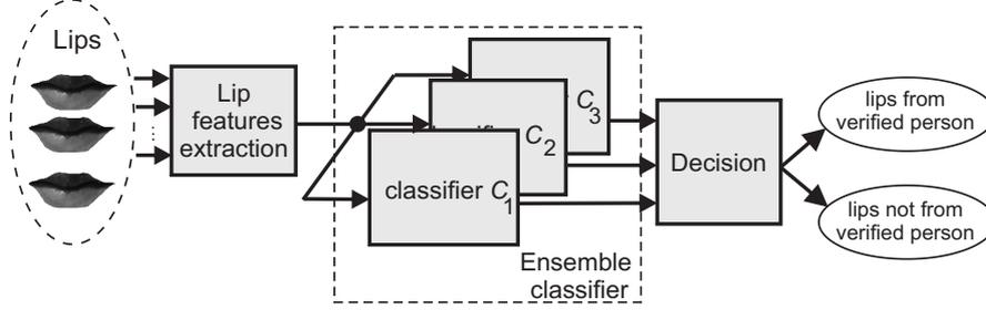
Fig. 6. The general structure of proposed classifier.
