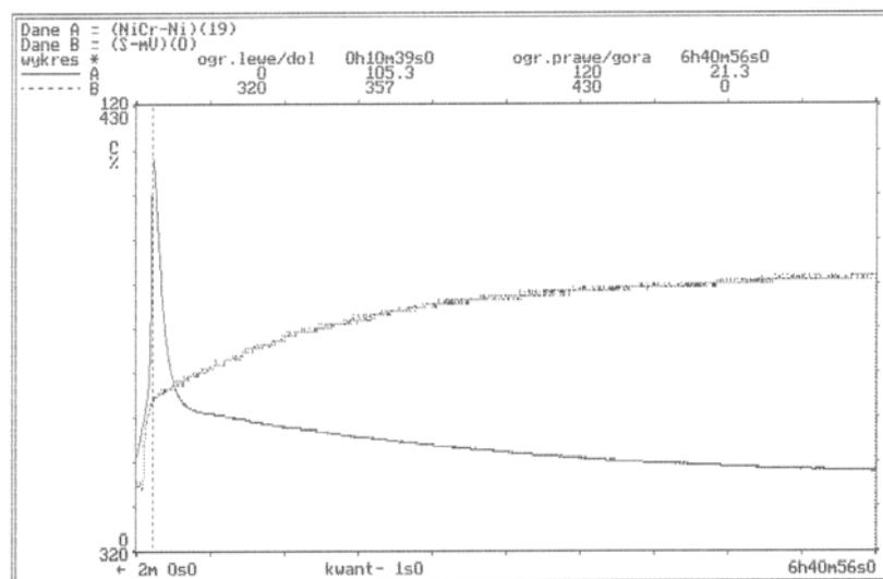
Fig.2. Change of the polymerisation temperature and linear contraction in course of time for Palacos R cement with Al<sub>2</sub>O<sub>3</sub> (powder of 10-20 µm granulation) into metal mould at initial temperature 37 °C.
