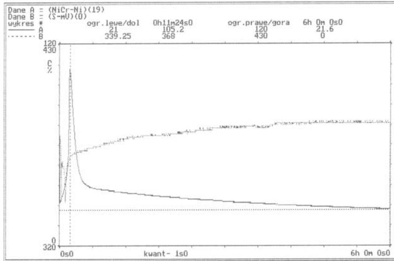
Fig.3. Change of the polymerisation temperature and linear contraction in course of time for Palacos R cement with  $Al_2O_3$  (powder of 0,3  $\mu m$  fraction) into metal mould at initial temperature 37  $^{\circ}C$ .
