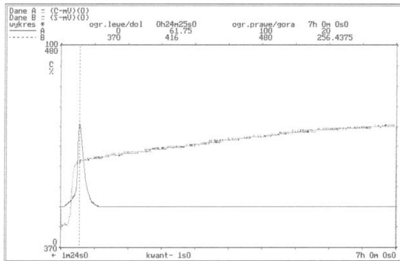
Fig.1. Change of the polymerisation temperature and linear contraction in course of time for Palacos R cement with Al<sub>2</sub>O<sub>3</sub> (powder of 10-20 µm granulation) into metal mould at initial temperature 19 °C.
