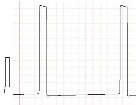
Fig.12. The 300 \mu V response of recorder no. 4, lead I, 20 mm/mV, good fulfillment of requirements.
