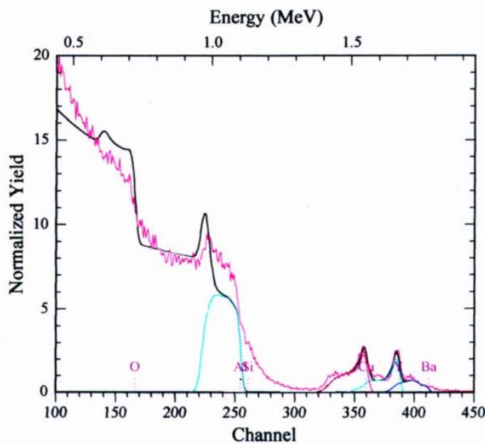
Fig.2. Experimental curves obtained by the RBS method for sample:  $\text{SiO}_2 - \text{Al}_2\text{O}_3$  layer ( $1000^\circ\text{C}$ ) - YBCO layer. Temperature of the YBCO layer synthesis: about  $800^\circ\text{C}$ ; ratio  $\text{Y}(\text{tmhd})_3 : \text{Ba}(\text{tmhd})_2 : \text{Cu}(\text{tmhd})_2 = 1 : 1,75 : 2,25$ ; synthesis time: 30 min.
