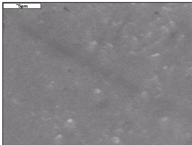
Fig.4. Surface of the YBCO layer synthesized at 800<sup>0</sup>C on quartz glass covered with Al<sub>2</sub>O<sub>3</sub> (1000<sup>0</sup>C). Molar ratio Y(tmhd)<sub>3</sub> : Ba(tmhd)<sub>2</sub> : Cu(tmhd)<sub>2</sub> = 1 : 2,25 : 2,36. Synthesis time: 15 min.
