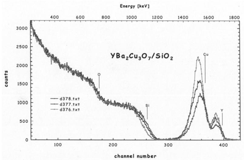
Fig.1. Experimental curves obtained by the RBS method for sample:  $\text{SiO}_2$  - YBCO layer. Temperature of the layer synthesis: about  $840^\circ\text{C}$ , ratio  $\text{Y}(\text{tmhd})_3 : \text{Ba}(\text{tmhd})_2 : \text{Cu}(\text{tmhd})_2 = 1 : 2 : 3$ , synthesis time: 30 min.
