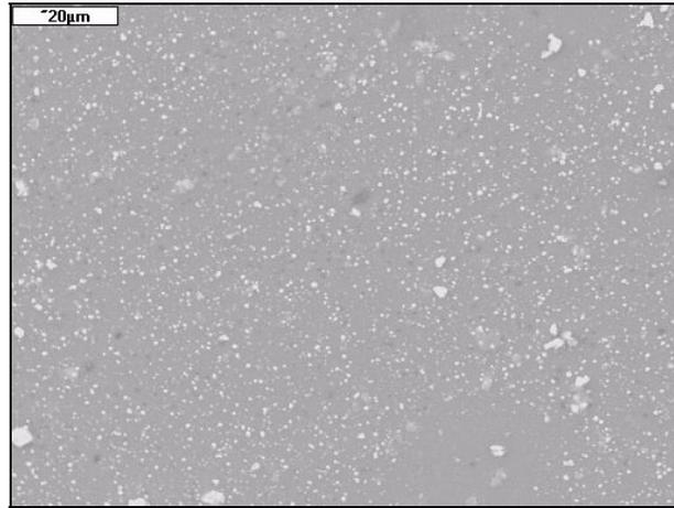
Fig.3. Surface of the YBCO layer synthesized at 870<sup>0</sup>C on quartz glass. Molar ratio Y(tmhd)<sub>3</sub> : Ba(tmhd)<sub>2</sub> : Cu(tmhd)<sub>2</sub> = 1 : 2,2 : 2,3. Synthesis time: 30 min.
