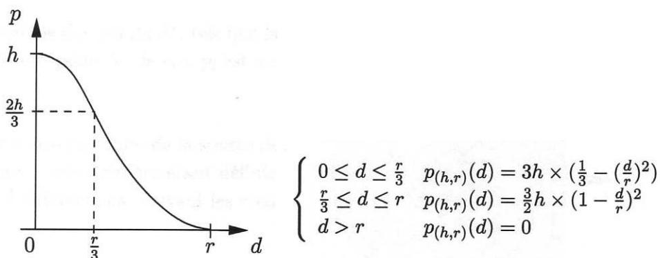
Then we distribute such potential sources along a line in the parametric space. We note that these sources may have different parameter values ( $h$  and  $r$ ) as shown in figure 4.
