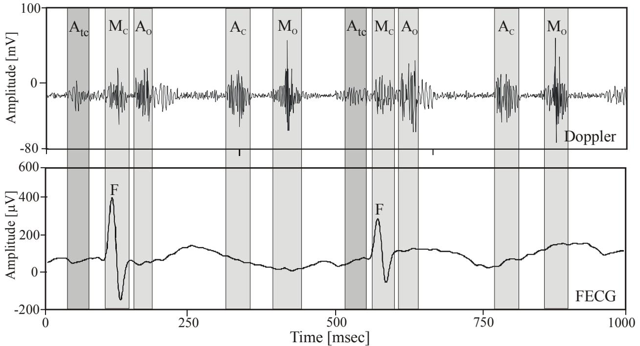
Fig.1. Signal of mechanical and electrical activity of fetal heart recorded simultaneously. M<sub>C</sub> and M<sub>O</sub> – atrioventricular valve closure and opening, A<sub>C</sub> and A<sub>O</sub> – semilunar valve closure and opening, A<sub>tc</sub> – atrial activity, F – fetal QRS complexes.
