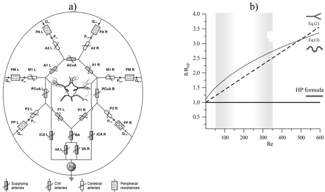
Fig. 4. a) Electric model of the Circle of Willis; b) Sketches of equations (2) and (3) in the dynamic state and within the range of  $Re$  number typical for physiology, for exemplary values  $a/a_K = 0.36$  and  $d/l = 0.1$ .
