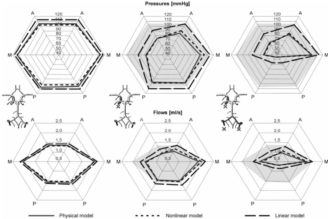
Fig. 5. Comparison of results of experiments (physical model) and blood flow simulations for the nonlinear and linear model in conditions: I - patency of all supplying vessels, II - occlusion of the left ICA, III – complete occlusion of the VBA system and the left ICA. Physiological pressure and flow rate values in cases II and III are highlighted
