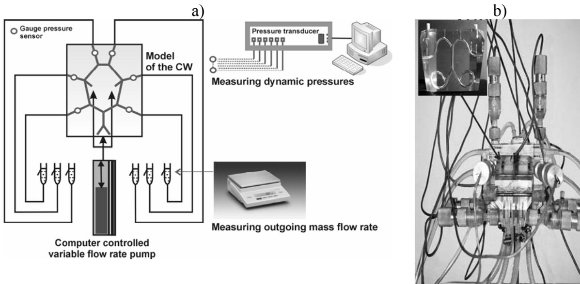
Fig. 3. a) Experimental set-up for measuring pressure and flow rate distributions;
