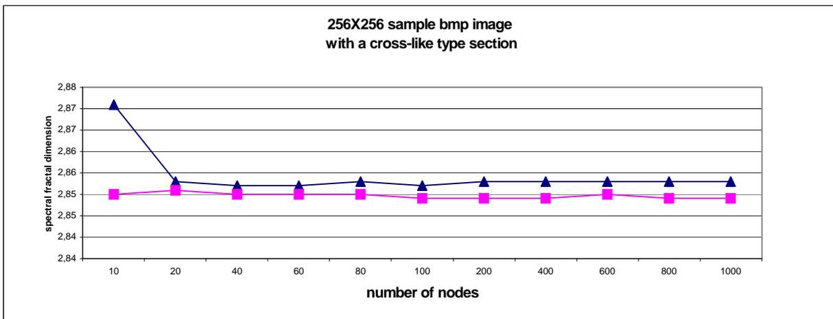
Fig. 4. Sample graphs presenting the results of testing calculations of spectral fractal dimension values  $D_s$  for selected *bmp* images of cross-like shapes of power spectrum sections. Numbers of nodes have been equal to 1000, and two types of spacing have been chosen: linear shown as triangles and logarithmic shown as squares (see the text for details).
