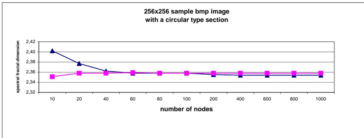
Fig. 5. Sample graphs presenting the results of testing calculations of spectral fractal dimension values  $D_s$  for selected *bmp* images of circular shapes of power spectrum sections. Numbers of nodes have been equal to 1000, and two types of spacing have been chosen: linear shown as triangles and logarithmic shown as squares (see the text for details).
