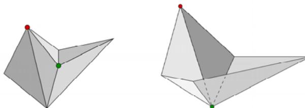
Fig. 6. Left: A convex vertex and its saddle neighbour. Right: A convex vertex and its concave-fan neighbour
