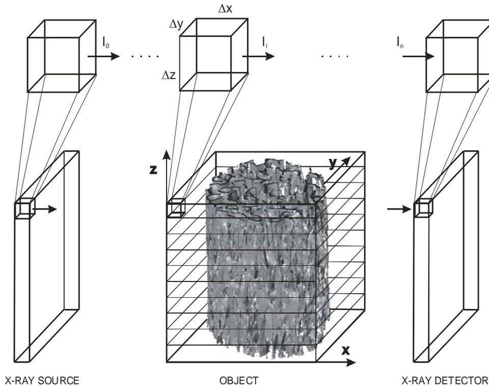
Fig. 2. The geometry of the simulation space and the rules for the numerical estimation of X-ray attenuation
