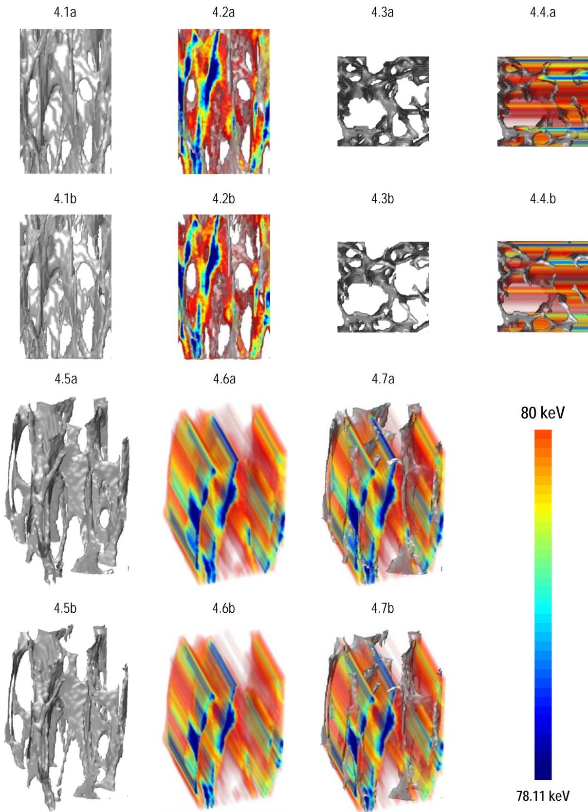
Fig. 4. The sample geometry and the distribution of X-ray radiation intensity during the propagation through the sample.
