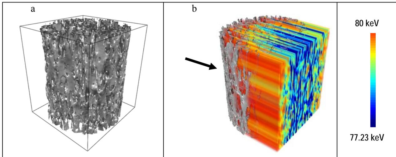
Fig. 3. Three-dimensional images of the virtual specimen, a) surface rendering of the bone microstructure model; b) superposition of the bone geometry and the visualization of X-ray radiation computed during propagation through the virtual specimen.
