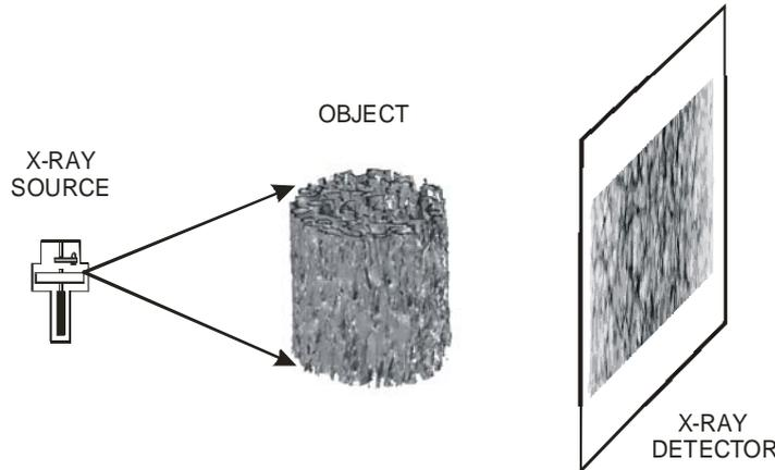
Fig. 1. The measurement process of the transmission tomography for single projection.
