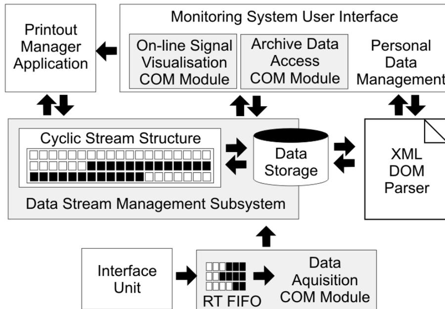
Fig. 3. Software architecture of centralized neonatal monitoring system
