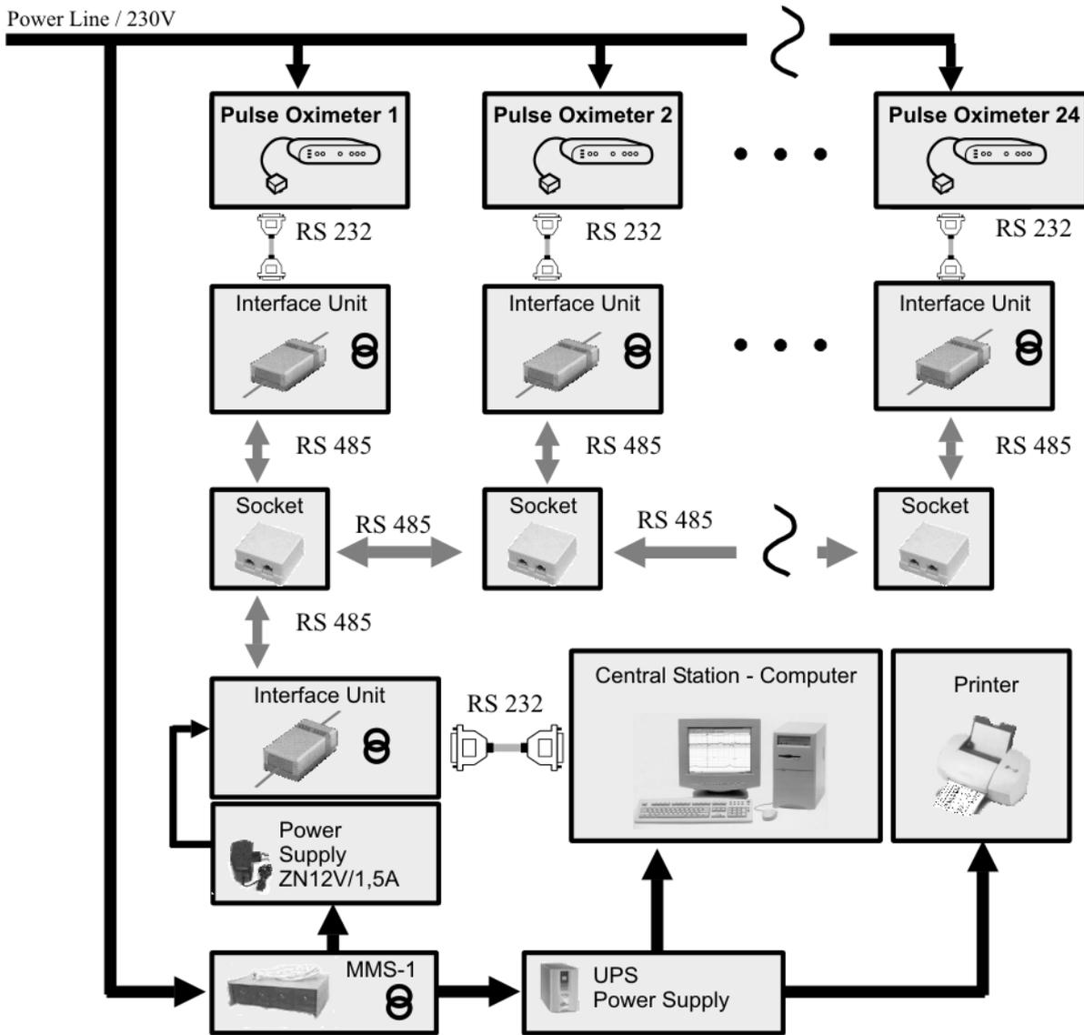
Fig. 1. Hardware structure of neonatal monitoring system
