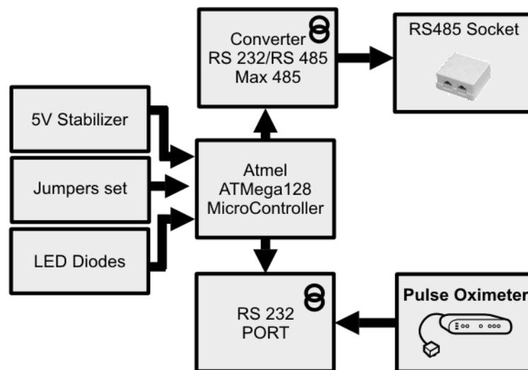
Fig. 2. Hardware structure of interface unit
